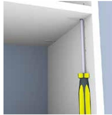
**STEP 3.** Use phillips screw driver no. 2 to unlock each fixed cam by inserting the screw driver and turning it 180 degrees or so the flat edge of each screw is facing the panel.
